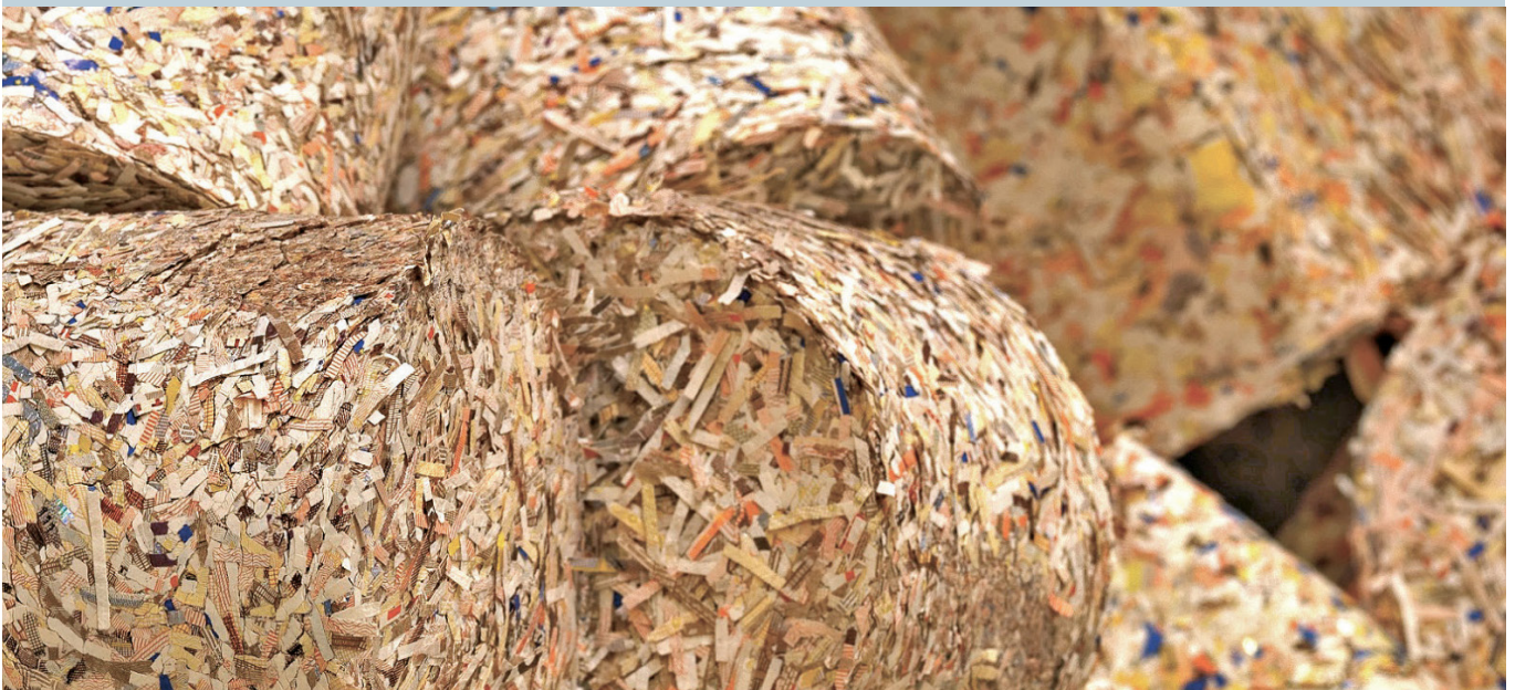
Photo 3. Briquettes of shredded banknotes
