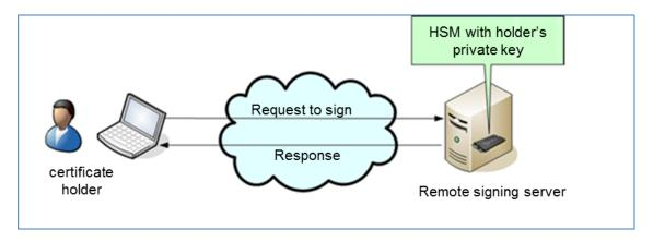
The signature client could be a desktop application or a third application that invokes the signing server by software interfaces.
